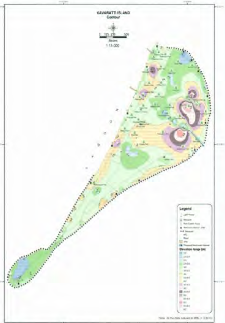
Fig.2.4.1.1 Map showing the contour elevation of Kavaratti island which ranges between 0.5 and 6 m above msl. High elevation is noted on the north-western part of the island.
