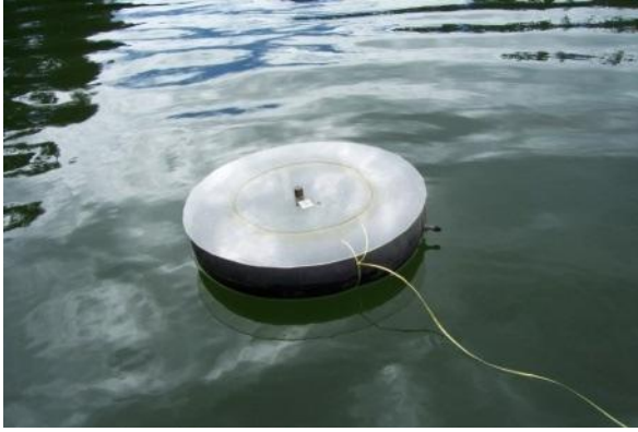
Fig. 3.3.1 Sampler deployed for collection of water to air fluxes of methane
