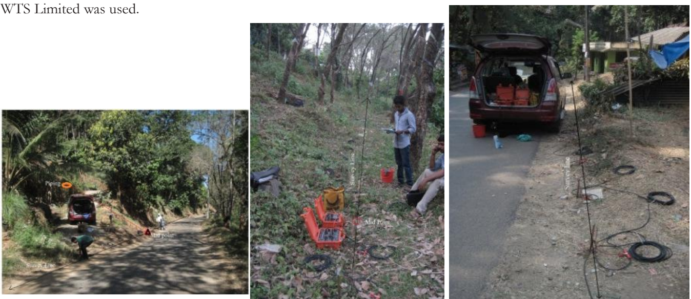
Fig. 1.10.4 The Electrical resistivity survey conducted at Idukki and Kannur districts.
