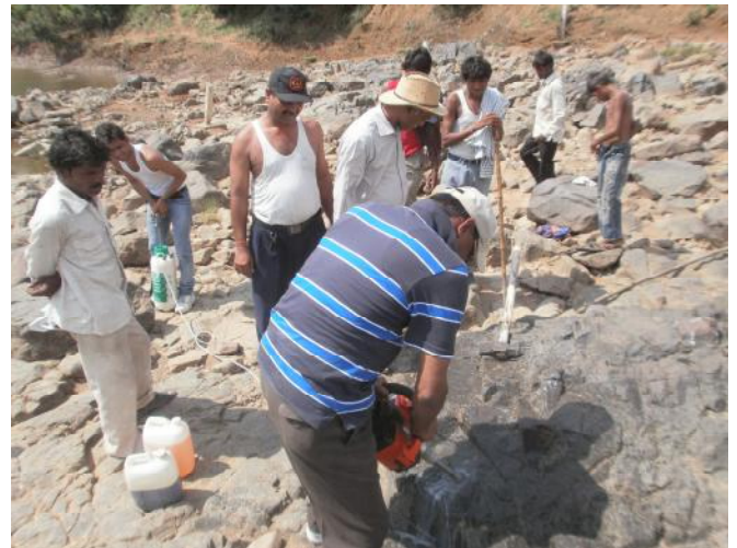
Fig. 1.2.1 A picture showing drilling for the collection of oriented cores from the Bijawar mafic volcanic flow in the Ken river section near Bhusor village
