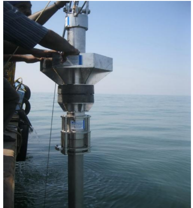
Fig. 2.2.2 Piston corer being operated for collection of sediment cores
