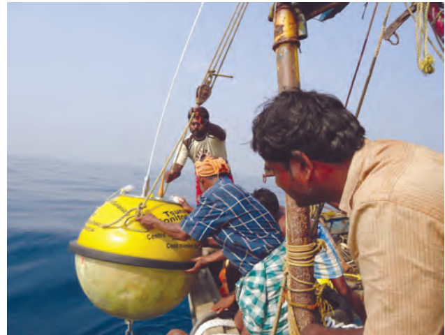
Fig. 2.3.2.1 Deployment of wave rider buoy off Valiathura at 30 m depth
