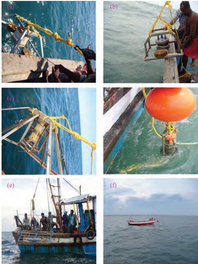
Fig.1.3.2.2 Deployment of equipments in progress: (a) Directional Wave Gauge, (b) Non-Directional Wave Gauge, (c) Acoustic Doppler Current Profiler (d) Recording Current Meter (e) Sediment trap assembly (f) A deployment site with the watch & ward team on duty
