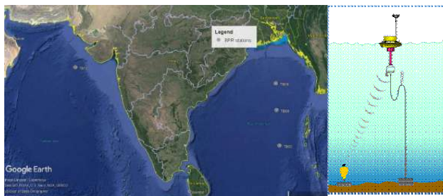
Fig. 2.11.1: Study area (a) Bottom Pressure Recorder (BPR) locations and (b) Anchored BPR and mooring for surface buoy
