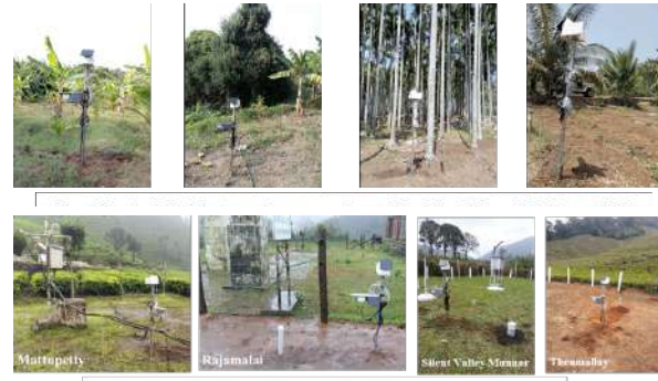
Fig. 4.1.2: Snapshots of the continuous profile soil moisture sensors installed in the Attappadi CZO
