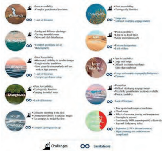
Fig. 3.5.10.2: Illustration showing region-wise challenges and limitations in identifying and quantifying the submarine groundwater discharge.
