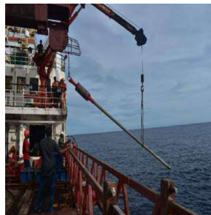
Fig. 2.7.4: Core sampling using Gravity core.
