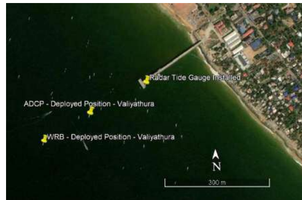
Fig. 2.3.1: Instruments installed/deployed off Valiyathura, Trivandrum
