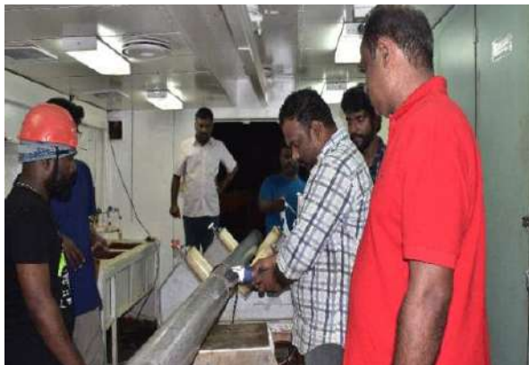
Fig. 2.7.5: Subsampling of the collected cores.
