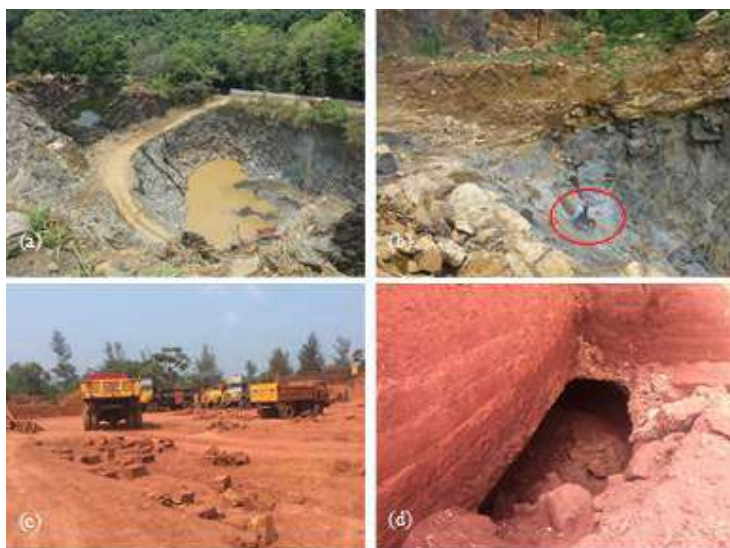
Fig. 4.5.2: Selected scenes from the study area. (a) Pit lake developed in a hard rock quarry in the Periyar – Chalakudy river basin. (b) Labourers at work (see the encircled portion) on a quarry slope without any protective measures. (c) Laterite quarrying in the Netravati – Gurupur river basin. (d) Tunnel erosion discovered at the active quarry of Navur, Netravati – Gurupur river basin.
