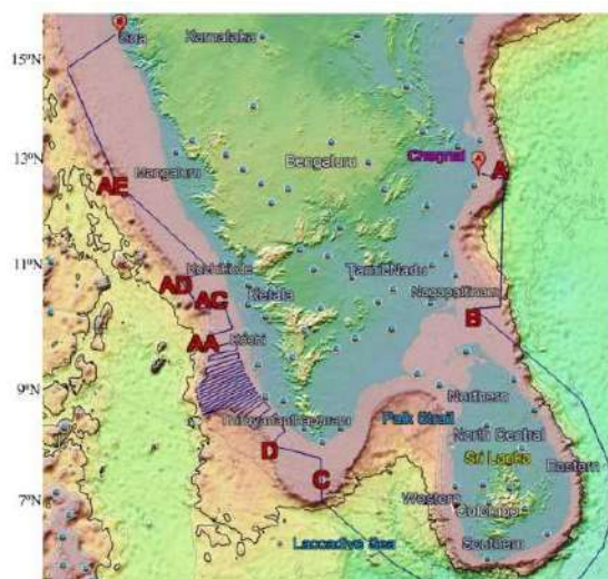
Fig. 2.8.1: High resolution CTD and LISST measurements along the transects in the south west coast of India (Transect names labelled in English alphabetical order from south to north).
