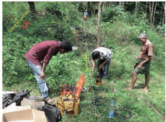
Fig. 1.10.3 Electrical resistivity survey at Kottathalachimala, Kannur
