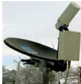
Fig. 1.2.4.1 Disdrometer used for rain drop size measurements in CESS. correlation (0.7) between the theoretical derivation and actual measurements.
