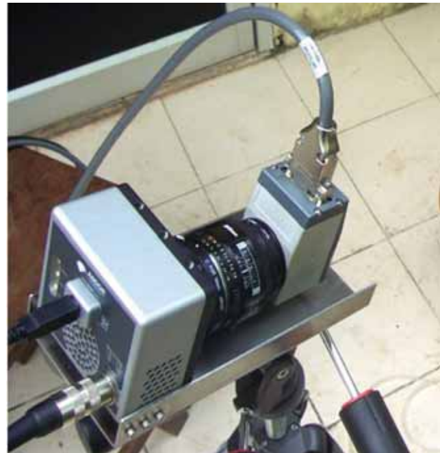
Fig.3.5.2.1 The multi-spectral imaging system developed in Biophotonics Laboratory for vegetation studies
