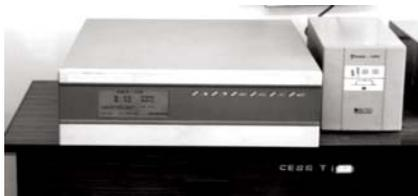
Fig. 1.2.2.1 CO analyzer (Monitor Eu-
