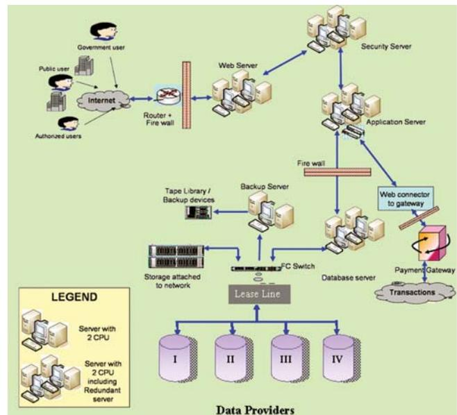
Fig. 3.6.6.1 Schematic diagram of the spatial data infrastructure
