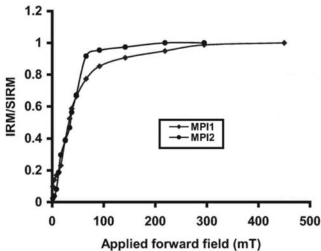
Fig. 1.1.4.2 Typical IRM acquisition curves of the pottery samples from Mayiladumparai, Tamilnadu
