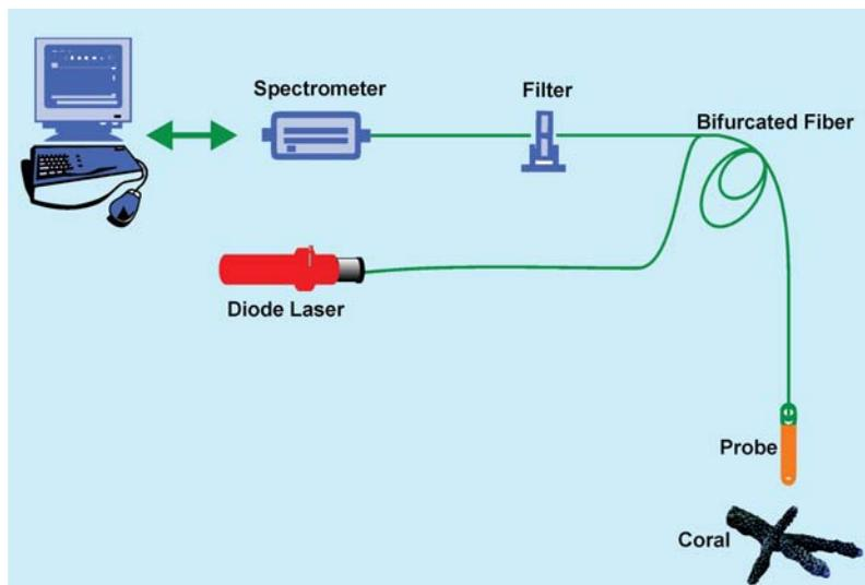
Fig. 1.3.4.1 Schematic diagram of the portable fiber optic fluorosensor
