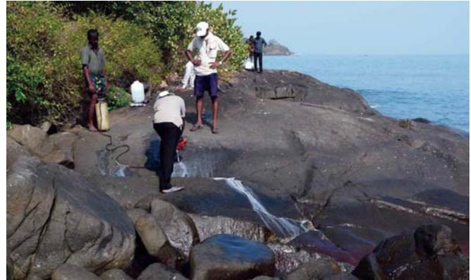
Fig. 1.1.3 .2 Drilling for collecting oriented core samples for palaeomagnetic study in South Islands of the St Mary's islands during a joint fieldwork by the Indian and French Collaborators
