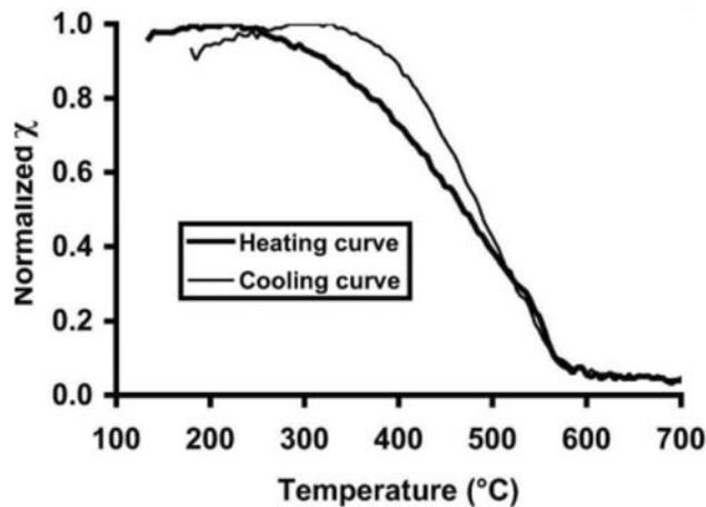
Fig. 1.1.4.1 Temperature dependent magnetic susceptibility of sample MPI-1 from Mayiladumparai, Tamilnadu
